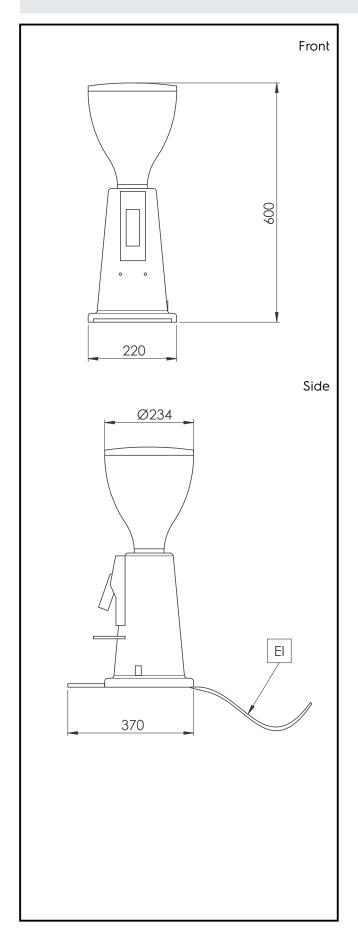
Coffee System Grind on-demand Coffee Grinder Coffee Grinder, Flat 75 mm
